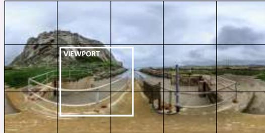
HEVC motion-constrained tiles with server-controlled sub-streams
